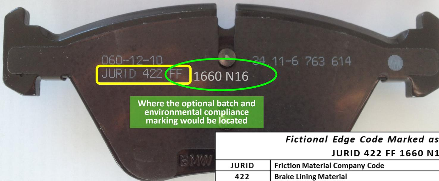
Where the optional batch and environmental compliance marking would be located
